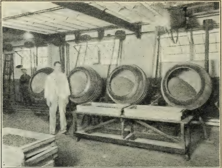
FIG. 35.—Making "sugar-coated peanuts," known as "burnt peanuts" by the trade. Note the steam coils around the outside of the revolving pans
